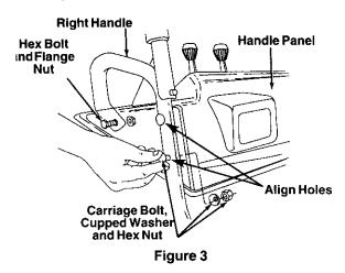
Attach the handle panel to the handle with two carriage bolts, cupped washers (cupped side against the handle panel) and hex nuts on each side. See Figure 3. You will find these fasteners in group B of the hardware pack. Align the contour of the carriage bolt head with the handle. Tighten the hardware.
